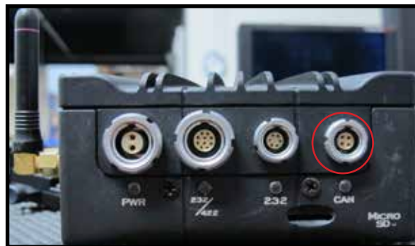
Figure 4.2a Connect from Wired port on THC to CAN port on 6-axis box (can also use 232 or 232/422 ports).
