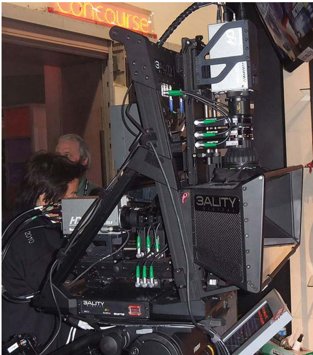
3ality rig with a pair of Ikegami HDL-51 cameras. Photo by Steven Bradford.
