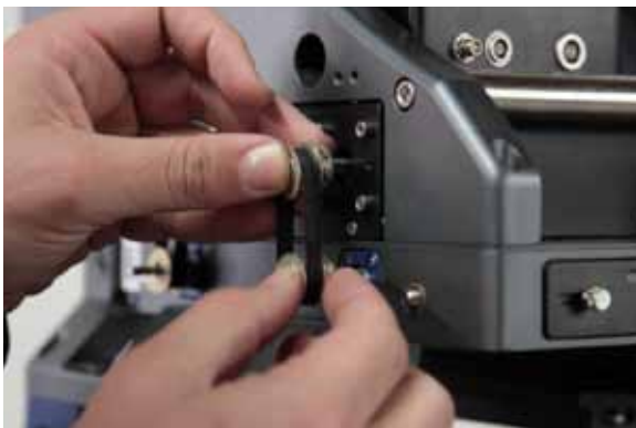
Slide top pulley and belt over lower pulley and push top pulley towards the rig.
