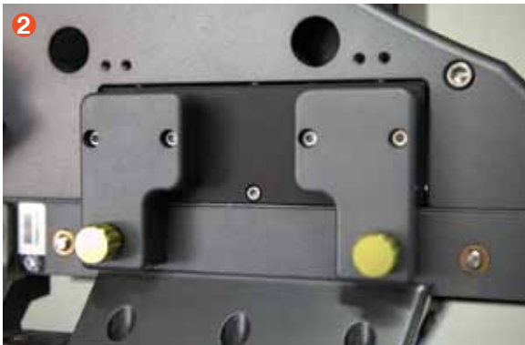
2 Using a .050" allen key, remove the moco plate knobs.
