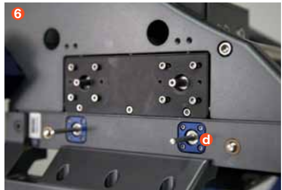
6 Check lead screw shafts (d). If there are any burrs, remove them by using fine sandpaper.
