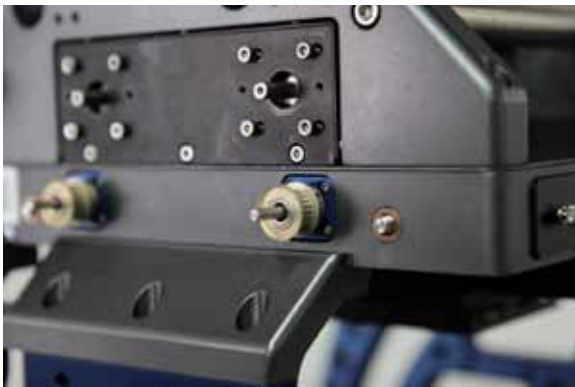
Slide new pulley over bushing. Be sure the rig side of the pulley is flush with the bushing and tighten using a 1.5mm allen key.
