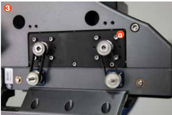
3 Using a 7/16" allen key, remove the pulley covers. Loosen all eight screws around top pulleys (a).
