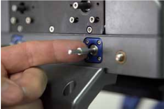
Slide supplied bushing onto the lead screw shaft.
