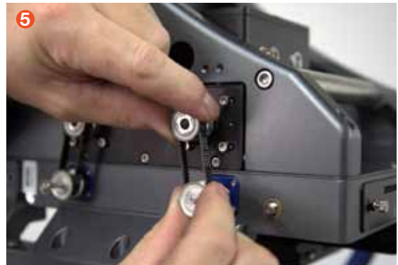
5 Once all pulleys are loose, pull both pulleys at the same time to remove pulleys and belt.
