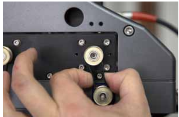
Slide top pulley to the center of the motor box. Apply slight pressure and lock down the retainer bolts. Belt should have a slight give.
